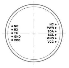
\* Note: Two VCCs are connected internally.
